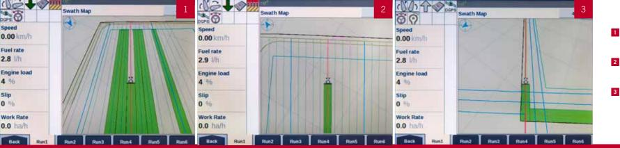
AccuTurn<sup>™</sup> for automatic and comfortable turns the end of a pass
