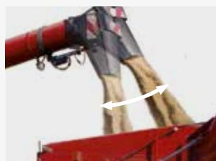
The pivot spout option is operated with the multi-function handle and directs the grain stream into the grain cart, filling it without spillage to maximum level.
