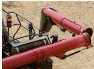
The 8.8 m and 10.4 m unloader tube is available as a foldable version for easier transport on the road and for easier manouevring in sheds for storage.
